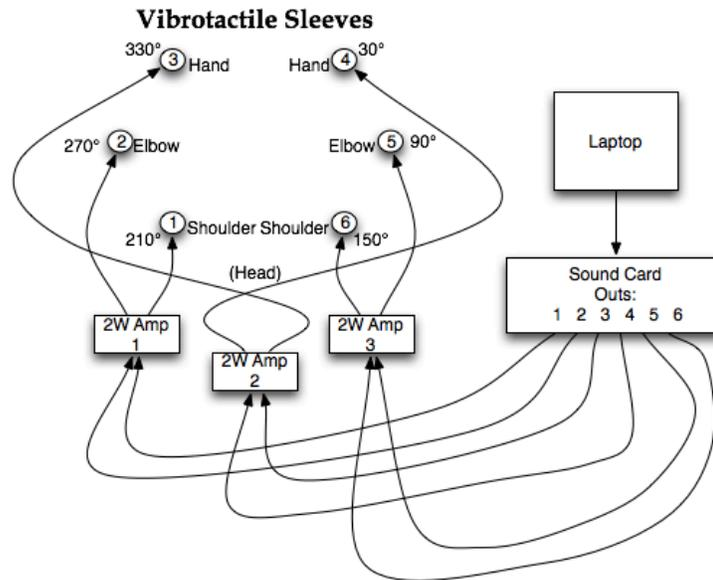
Figure 1: Vibrotactile Sleeves with 6-channel actuator configuration and signal flow chart.
