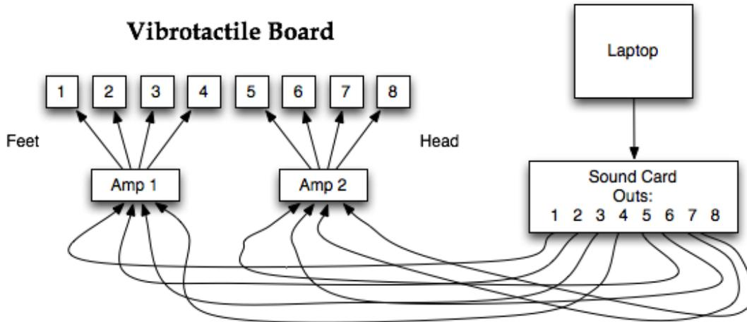
Figure 2: Vibrotactile Board with 8-channel actuator configuration and signal flow chart.
