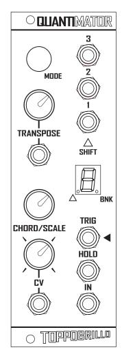
**OUTS 1-3**- 1V/oct quantized control outputs to control stuff. output range is 0-5V [5 octaves].
