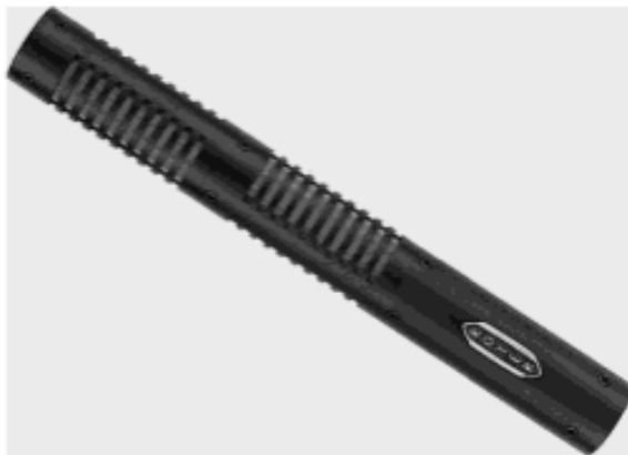
Figure 6-23 A stereo pair of matched ribbon mics mounted one above the other in a single casing. The two ribbons' pickup patterns are 90 degrees off-axis from each other.
