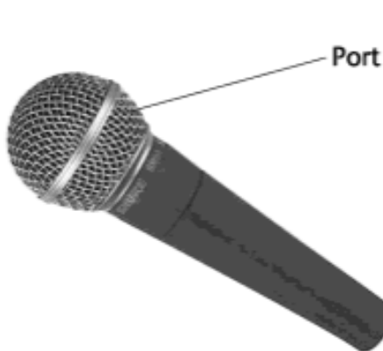
Figure 6-6 Microphone with single entry port. Note: This figure and Figure 6-7 indicate the positions of the ports on these mics. The actual ports are concealed by the mic grille.
