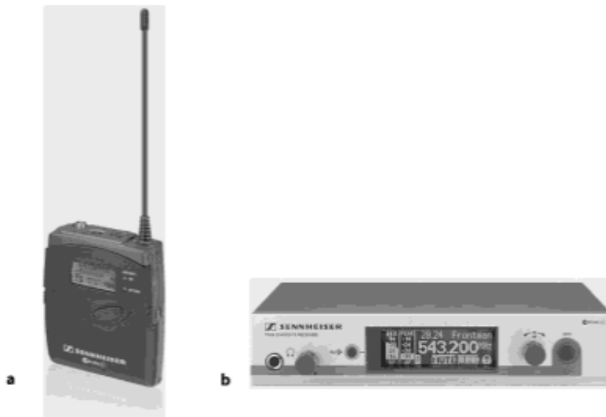
Figure 6-28 Wireless microphone system. (a) Pocket transmitter. Features include: multiple UHF frequency selection; long-range transmission; illuminated graphic display; auto-lock to avoid accidental change of the selected frequency; mute function; and wireless synchronization of transmitters via infrared interface from the receiver. (b) Receiver. Features include: diversity reception (see “Diversity Reception” later in this section); illuminated graphic display also showing transmitter settings; automatic frequency scan to search for available frequencies; Ethernet port; and integrated equalizer and soundcheck mode.
