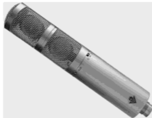
Figure 6-24 Stereo microphone with one rotating capsule. The upper capsule in this model can rotate 270 degrees horizontally; the lower capsule is stationary. Two three-way switches control the polar response, high-pass filtering, and -10 dB pad for each capsule.
