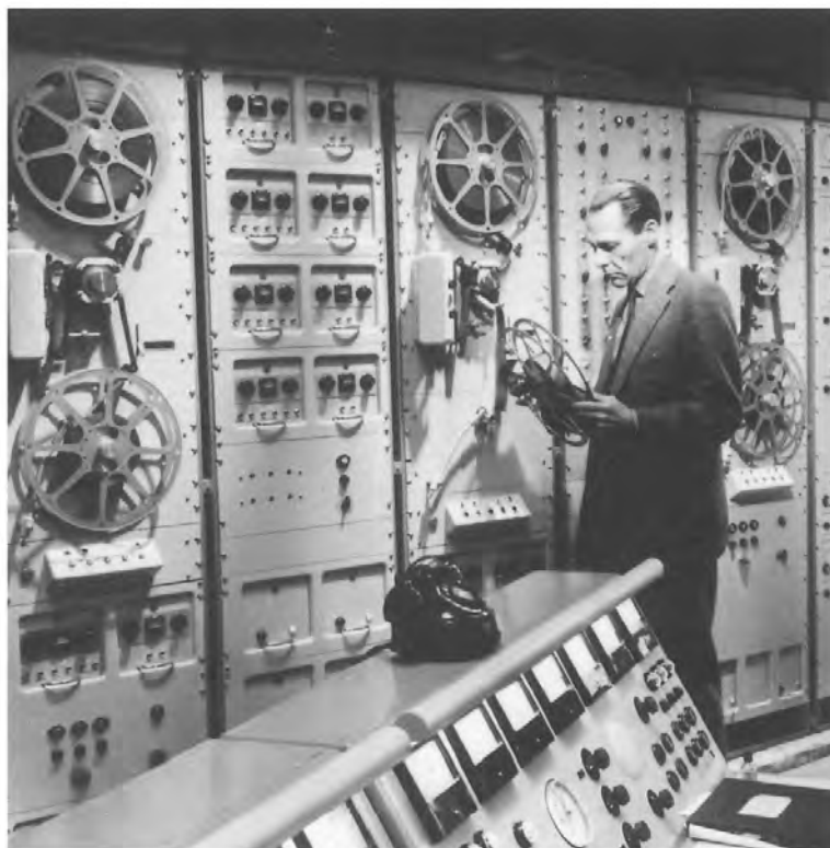
Figure 8.2 Playback and spatial switching system in the Philips Pavilion control room based on 35 mm sprocketed magnetic tape.
