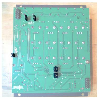
Single Pressure Points with no BRAINS attached: Note all the "Close 4 Master" locations are closed, as well as the Expand headers.
