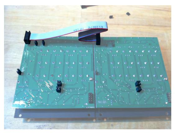
Two Pressure Points, chained: Note that the "Close 4 Master" headers are closed on the first unit (will be on the right when installed in the case). For three or four Pressure Points, use 4-header CHAIN cable and leave "Close 4 Master" headers open on all units but the master (rightmost when installed/leftmost from behind). Also, note the jumpers on the EXPAND headers.
