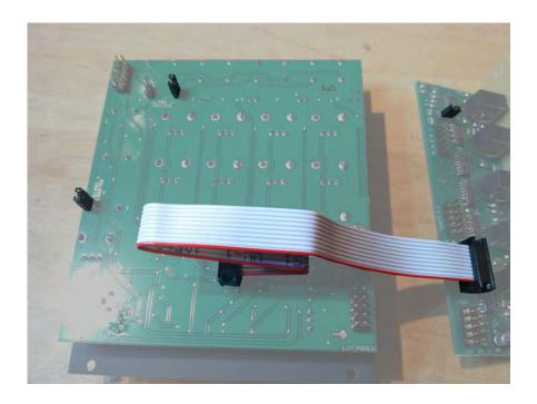
**BRAINS with a single Pressure Points:** Note the single open "Close 4 Master" header, the BRAINS cable connected from "Points 1-4" header to EXPAND header, and the jumper on BRAINS set to "1PP."
